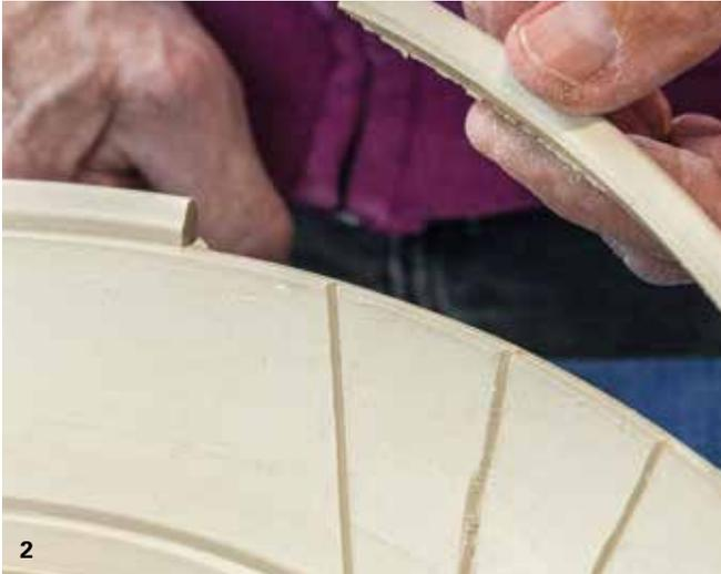
2 Make at least two passes with a single-edge razor blade to cut through the rim of the bowl.
